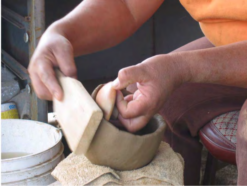
Figure 4. Modern paddle-and-anvil pottery production in Santa Catarina.
